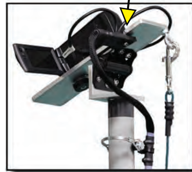
Camera firmly secures to mast Cables move with Camcorder
